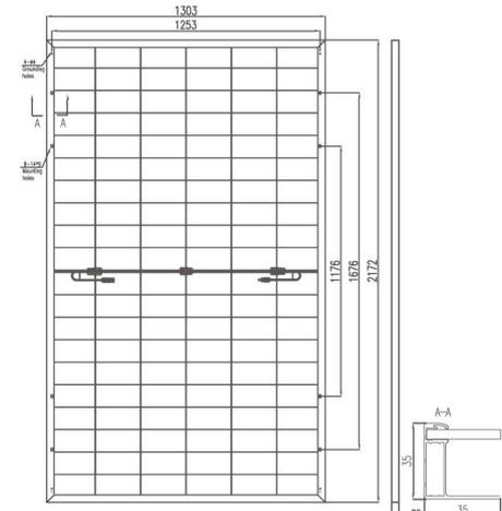
\*400mm mounting holes are only suitable for 6005-T6 aluminum frame
